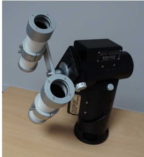
Figure 11 The C-DIMM can be mounted on an astronomical mount (shown here without its enclosure) to track stars during the night.
