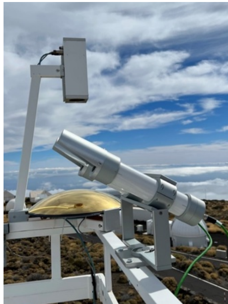
Figure 18 First version of the LWIR allsky camera and its gold coated mirror. The C-DIMM is also visible at the foreground of the picture. Image taken at the Teide Observatory (Izaña, Spain).
