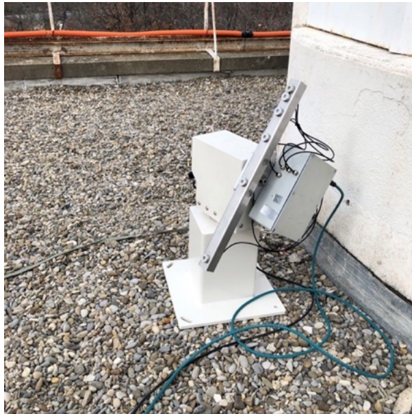
Figure 8 The SHABAR is a daytime turbulence profiler mounted on a tracking mount.
