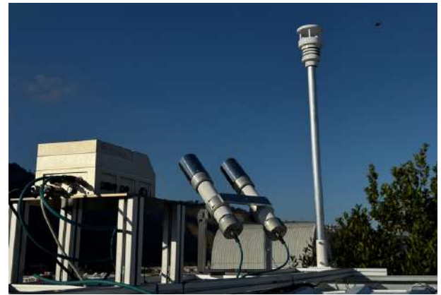
Sky Monitor : All in one instrument Standard configuration : Main Unit, C-DIMM & weather station + Optional Equipments
